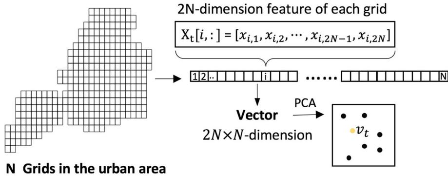
**Fig. 4** The characteristic of point  $v_t$  is captured by an  $N \times 2N$ -dimensional feature vector, where  $N$  indicates the number of grids in a region and  $2N$  is the number of features of each grid
